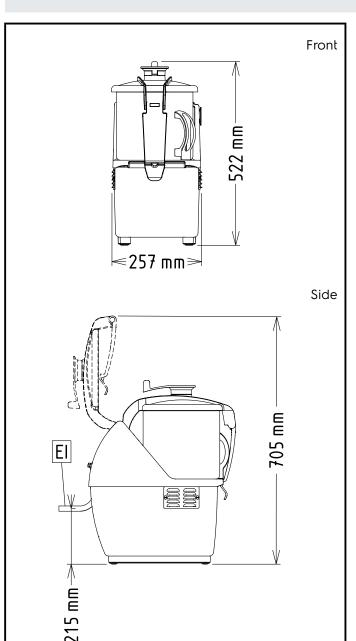
**Electric** Supply voltage: 380-440 V/3 ph/50/60 Hz Electrical power, max: 1.2 kW **Total Watts:** 1.2 kW Capacity:
